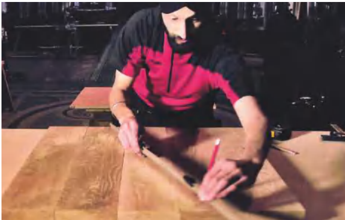
▲ Pic.4 Marking out the centre point on the timber, using the Trend flat lying trammel set to 350mm for the radius
